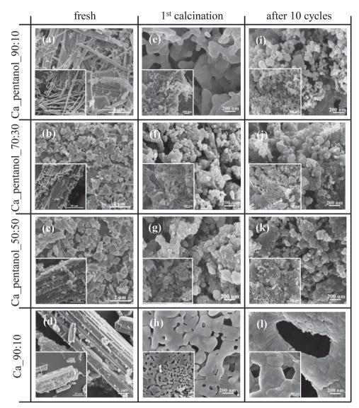
Figure 4. SEM images of Mg-supported calcium acetate: fresh, calcined and after being exposed to 10 carbonation-calcination cycles.
