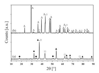
**Figure 6.** X-ray diffraction patterns: (a) calcined Ca\_pentanol\_50:50, (b) carbonated Ca\_pentanol\_50:50. The following compounds were identified: ( $\triangle$ ) – lime, CaO, ( $\triangle$ ) – calcite, CaCO<sub>3</sub>, ( $\spadesuit$ ) – portlandite, Ca(OH)<sub>2</sub>, ( $\square$ ) – periclase, MgO.
