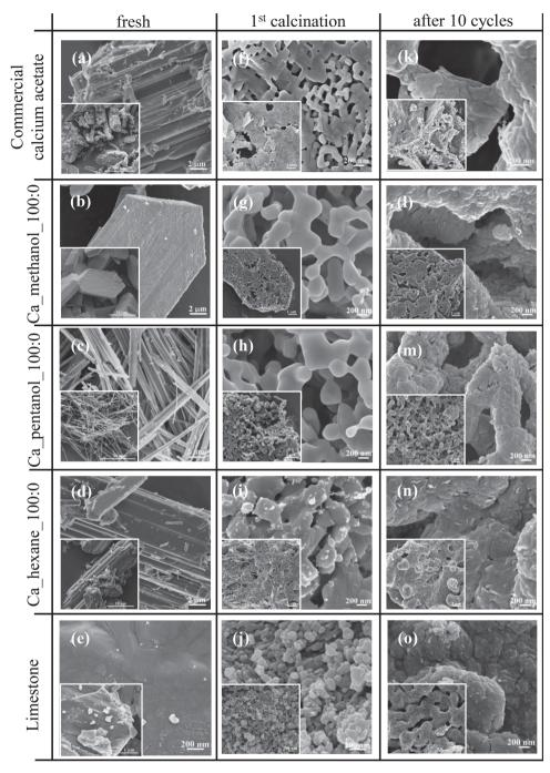
Figure 1. SEM images of pure, i.e., unsupported, calcium acetate: fresh, calcined and after being exposed to 10 carbonation-calcination cycles. The micrographs of calcined and reacted limestone were plotted for comparison.
