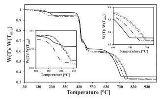
**Figure 2.** Normalized weight change as a function of temperature during  $N_2$ -TPD: (---) Ca\_methanol\_100:0, (--) Ca\_pentanol\_100:0, (--) Ca\_hexane\_100:0 and (---) commercial calcium acetate hydrate. The temperature ramp was 10 °C (min)<sup>-1</sup> with  $T_{min} = 30$  °C and  $T_{max} = 1000$  °C.
