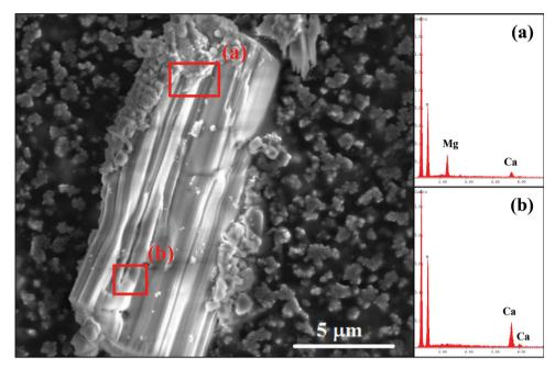
Figure 5. SEM image and EDX spectra obtained at different locations of Ca\_pentanol\_70:30.
